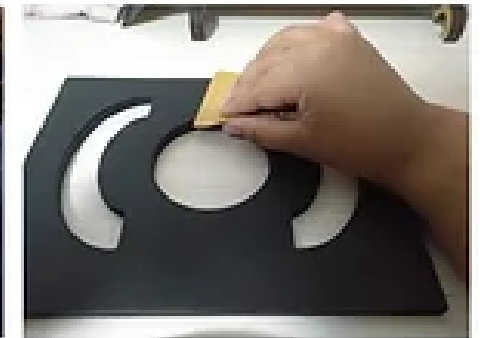
Smoothened the surfaces using sandpaper.
